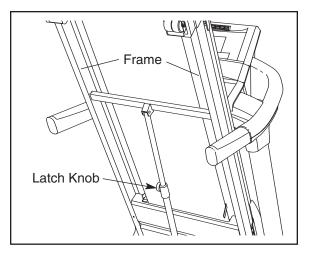
2. Hold the metal frame firmly with both hands, and lower it to the floor. CAUTION: To decrease the possibility of injury, do not lower the frame by gripping only the plastic foot rails. Do not drop the frame to the floor. Make sure to bend your legs and keep your back straight.
